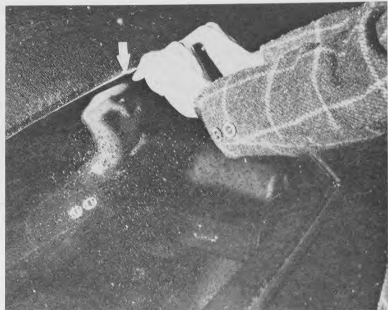
THE PROFESSIONAL WAY --All one has to do is slip between the window and the molding, and rip quickly. That will break the window out of its tracks. This usually happens to those who leave the window open slightly.
